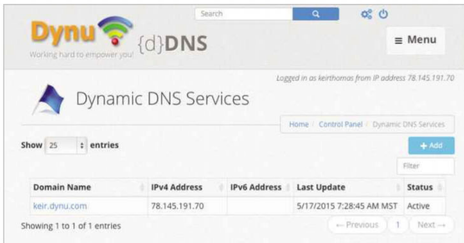
▲ A dynamic DNS service lets your local network have an actual hostname, like familyhub.dynu.com , at which it can always be reached
